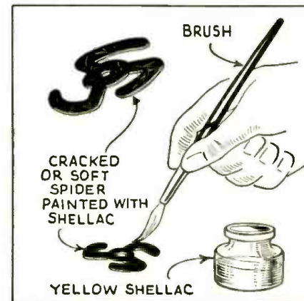
Fig. 5. An anti-rattle idea that increased loudspeaker life.
