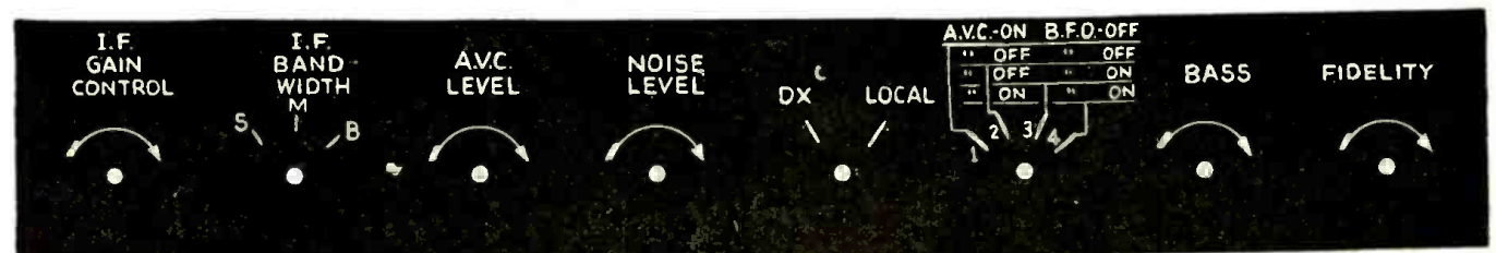
Fig. 9. Markings for the various controls on front apron of the chassis.
